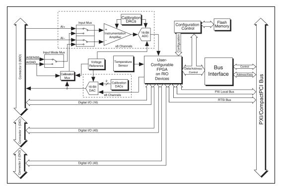
Figure 2-1. NI PXI-7831R Block Diagram
